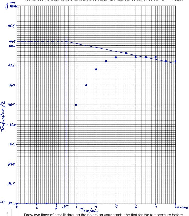
Draw two lines of best fit through the points on your graph, the first for the temperature before adding **FB 2** and the second for the temperature of the mixture after addition of **FB 2**. Extrapolate the lines to  $t = 2\frac{1}{2}$  minutes and determine the theoretical maximum temperature rise,  $\Delta T$ .
